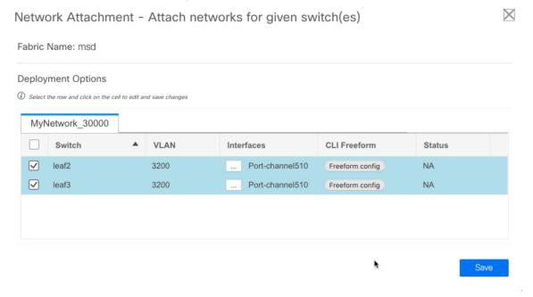
The **Interfaces** window lists interfaces or port channels. You can select interfaces/port channels to associate them with the selected network. These port channels connect the leaf switches to the ToR switches. The networks will be deployed on these port channels.
