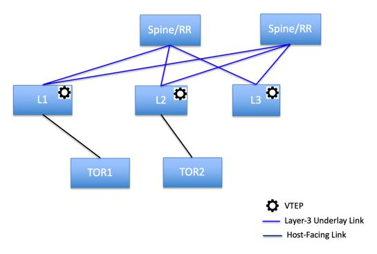
The following topology with ToR switches is not supported in DCNM:
