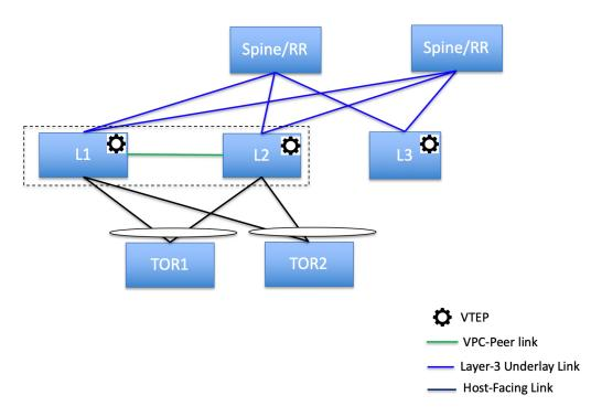
• ToR switches with port channels directly connected to the leaf switches. The L1 and L2 switches are connected as a vPC pair.
