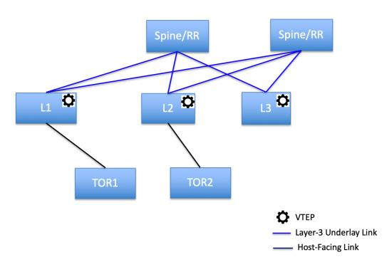
The following topology with ToR switches is not supported in DCNM:
