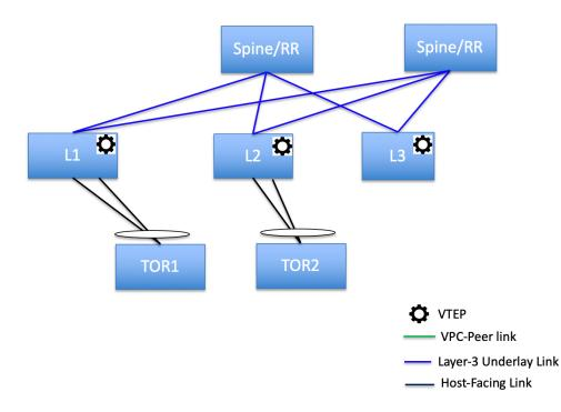
• ToR switches directly connected to the leaf switches. vPC pairs are not configured for the leaf or ToR switches.
