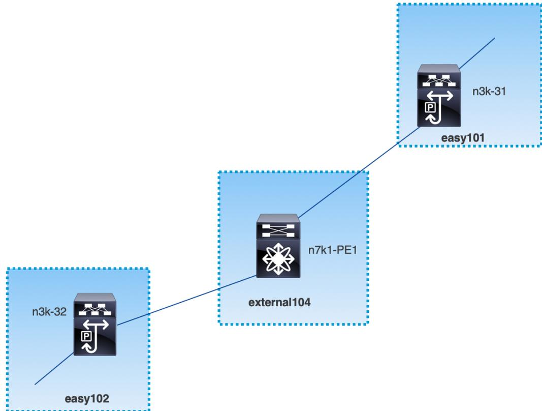
This topology shows only the border devices in the Easy Fabric and the core or edge router in the external fabric.
