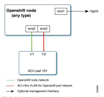
The first interface is used for the node network and the second one is used for the pod network. The second interface also carries Cisco ACI control plane traffic. A VLAN tagged subinterface can be configured on the second interface to carry the cluster's pod traffic and also the Cisco ACI control plane traffic.
