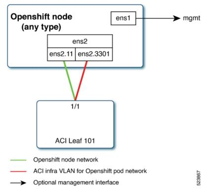
The node network and pod network are configured as VLAN subinterface of either bond0 or physical NIC. You can configure the server with additional VLAN(s) for management purpose or use the node network for management network. The design might be dependent on the server provisioning method (PXE or manual ISO boot).
