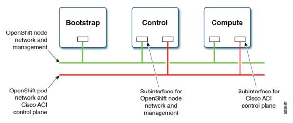
The first interface is used for the node network and the second one is used for the pod network. The second interface also carries Cisco ACI control plane traffic. A VLAN tagged subinterface is configured on the second interface to carry the cluster's pod traffic and also the Cisco ACI control plane traffic.
