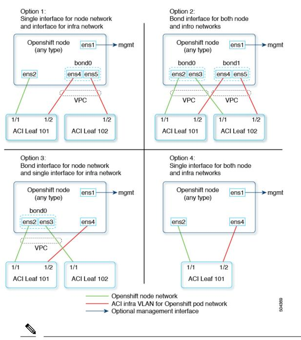
**Note** Node network is configured as VLAN subinterface of either bond0 or physical NIC. You can configure the server with additional VLAN(s) for management purpose or use the node network for management network. The design might be dependent on the server provisioning method (PXE or manual ISO boot).
