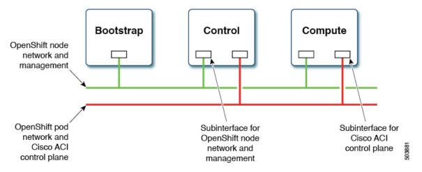
The first interface is used for the node network and the second one is used for the pod network. The second interface also carries Cisco ACI control plane traffic. A VLAN tagged subinterface is configured on the second interface to carry the cluster's pod traffic and also the Cisco ACI control plane traffic.
