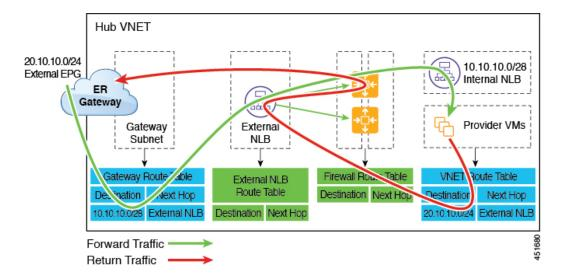
The following figure shows an example of a redirect for express route gateway to the provider EPG in the spoke VNet.
