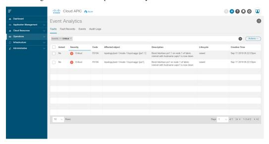
**Step 3** Click the **X** next to the Severity level to display Event Analytics information for all faults.
