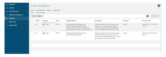
**Step 3** Click the **X** next to the Severity level to display Event Analytics information for all faults.
