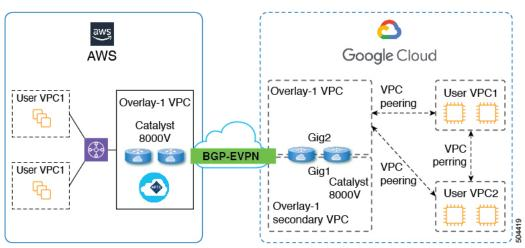
The following sections provide more information on the components that allow for inter-site connectivity using BGP-EVPN:
