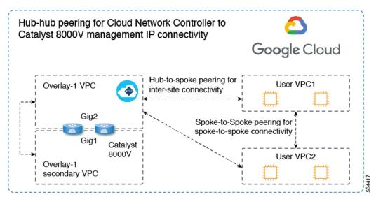
Cisco Cloud Network Controller automates configurations to exchange the routes between cloud sites in the following situations:
