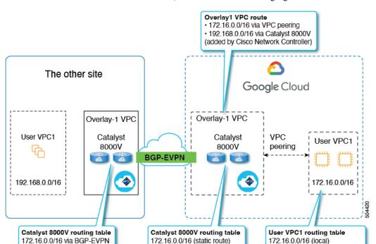
8000V routers in the other site through BGP EVPN. In this way, the Catalyst 8000Vs have the routes to reach the destination subnets in the other site, as shown in the following figure.
