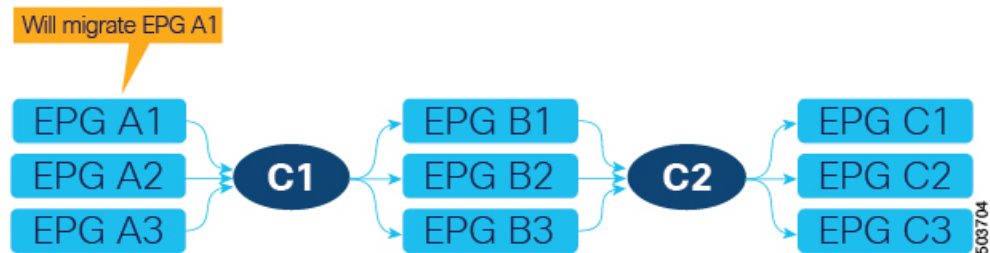
Figure 13: Prepare to begin EPG-to-ESG migration
