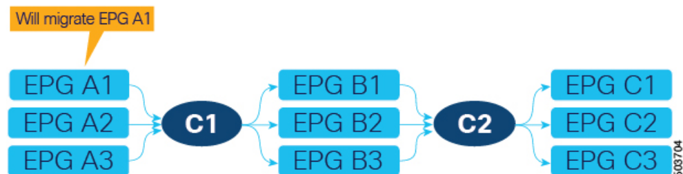
Figure 7: Prepare to begin EPG-to-ESG migration
