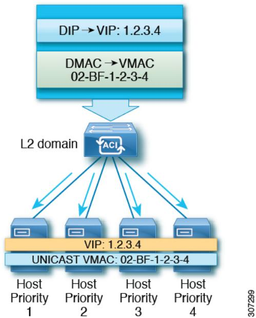
The use of a common MAC address would normally create a conflict, since Layer 2 switches expect to see unique source MAC addresses on all switch ports. To avoid this problem, Network Load Balancing uniquely modifies the source MAC address for outgoing packets. If the cluster MAC address is 02-BF-1-2-3-4, then each host's source MAC address is set to 02-x-1-2-3-4, where  $x$  is the host's priority within the cluster, as shown in the following figure.
