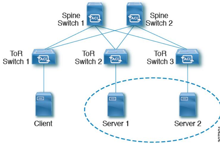
In this figure, Server 1 and Server 2 are in the MS NLB cluster. These servers appear as a single-host server to outside clients. All servers in the MS NLB cluster receive all incoming requests, then MS NLB distributes the load between the servers.
