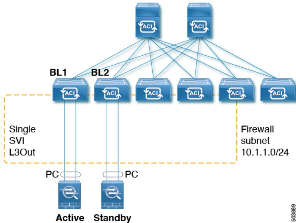
In this example, BL1 and BL2 are the border leaf switches on the fabric. Both border leaf switches are on the same SVI L3Out that connects to the external firewalls. Each firewall is connected to one of the two border leaf switches over a port-channel (non-vPC).
