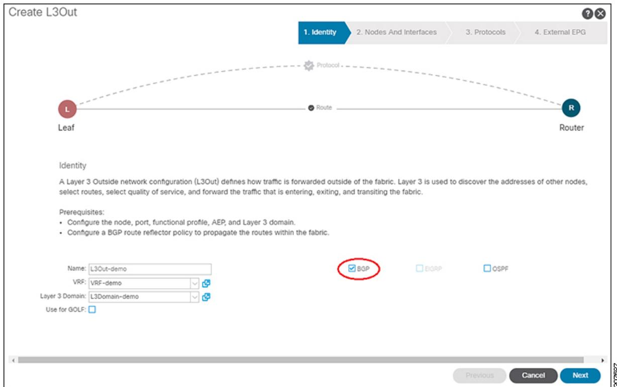
d) Continue through the remaining pages (**Nodes and Interfaces**, **Protocols**, and **External EPG**) to complete the configuration for the L3Out.
