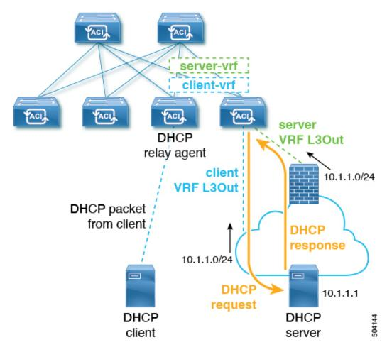
In this example scenario, the external DHCP server network is reachable in the ACI fabric via both the client and the server VRF instance. The DHCP relay packet is routed from the client VRF instance and sent via the client VRF instance L3Out. The source IP address in the DHCP relay packet is selected from the server VRF instance L3Out per the DHCP relay policy. The DHCP relay response from the server will be routed to the DHCP server L3Out, resulting in an asymmetric flow.
