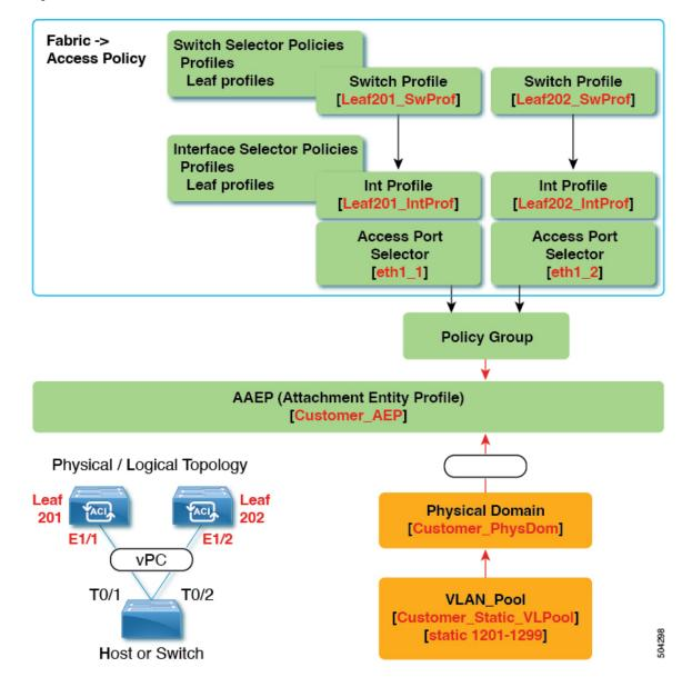
Figure 9: vPC With Different Leaf Switch Interfaces Across Two Leaf Switchs With Individual Profiles
