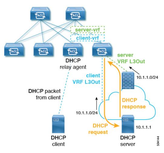
In this example scenario, the external DHCP server network is reachable in the ACI fabric via both the client and the server VRF instance. The DHCP relay packet is routed from the client VRF instance and sent via the client VRF instance L3Out. The source IP address in the DHCP relay packet is selected from the server VRF instance L3Out per the DHCP relay policy. The DHCP relay response from the server will be routed to the DHCP server L3Out, resulting in an asymmetric flow.
