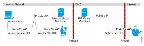
This is a schematic diagram of a split-horizon network topology.
