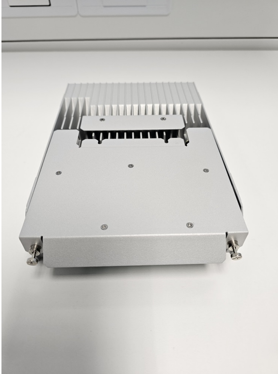
Figure 5: Slide the Replacement Fan Tray into the Module 10G
