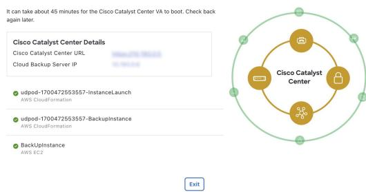
While the **Cisco Catalyst Center Configuration In Progress** window is displayed, record the backup server's IP address and the backup instance's stack name for later use. Your backup server password is a combination of the first four characters of the backup instance's stack name and the backup server's IP address without the periods.
