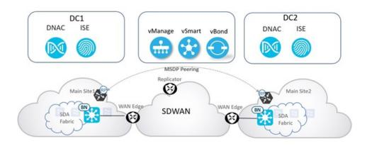
The financial vertical has native multicast enabled on the main, small, and mini sites. SD-Access native multicast relies on Source Specific Multicast (SSM) in the underlay; therefore, SSM configurations are configured on the fabric nodes, intermediate nodes, and SD-WAN WAN edges. Multicast Rendezvous Point (RP) is external to the SD-Access fabric. MSDP peering is enabled to communicate site-specific multicast sources to remote multicast RP. A replicator is configured in the SD-WAN WAN edge.
