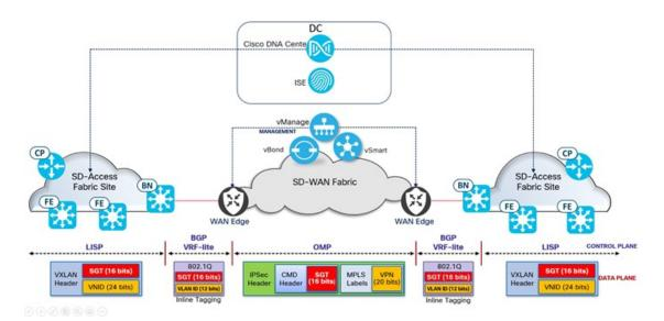
• After Cisco SD-WAN controllers are up and WAN edges are onboarded and managed by the Cisco SD-WAN controller, integration with the Cisco SD-Access network is achieved via IP transit L3 handoff on the fabric borders with VRF lite and eBGP.
