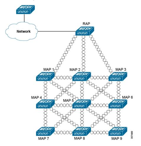
Both MAPs and RAPs can provide WLAN client access. However, typically, the location of RAPs is often not suitable for providing client access.
