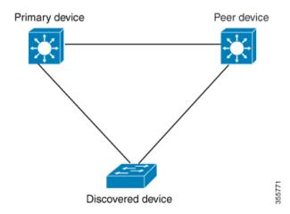
Cisco DNA Center configures the DHCP server on the primary device. Because Cisco DNA Center understands that the discovered device is connected to both the primary and peer devices, it configures two Layer 3 point-to-point connections when the LAN automation task is stopped. One connection is established between the discovered device and the primary device; the other connection is established between the discovered device and the peer device.
