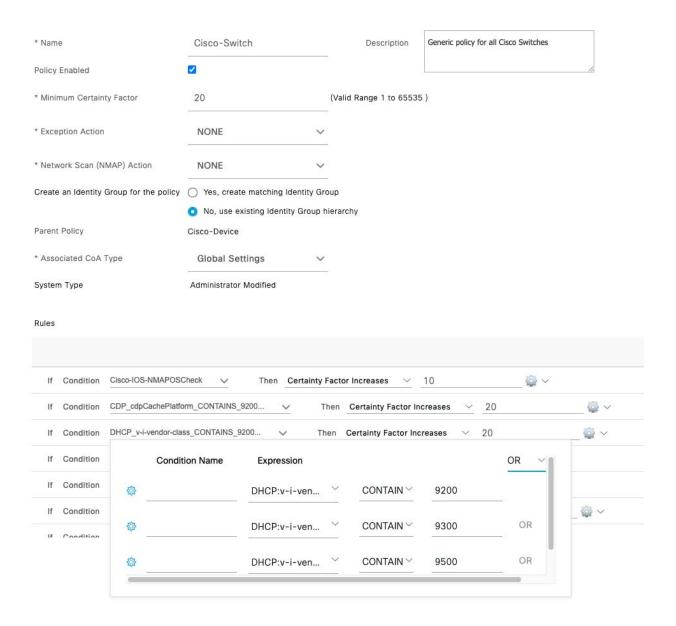
c) Create a new child policy for the supplicant device, under **Cisco-Switch** and apply the **CdpCachePlatform** and **V-I-Vendor-Class** conditions.
