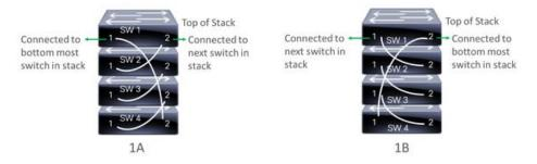
• Select a Top of Stack serial Number: From this drop-down list, choose the serial number of the top-of-stack switch, if you want to renumber the stack.
