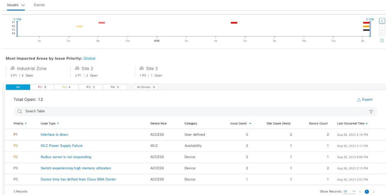
Furthermore, the Catalyst Center Assurance feature offers a system-guided approach to troubleshooting. It correlates information from various sources, such as device logs, network telemetry, and user reports, to determine the root cause of a problem. Once the root cause is identified, Assurance provides users with possible actions to resolve the problem effectively.
