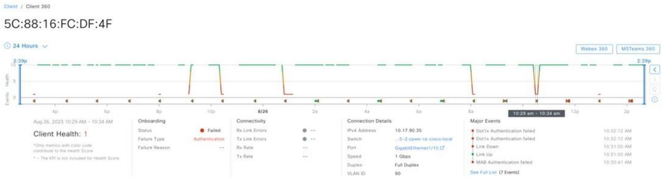
Client 360 also provides operators with insights into the neighbor switch information, link status, and utilization of a specific endpoint. The following figure shows link utilization of an endpoint on a selected time frame, aiding in network capacity planning and optimization.
