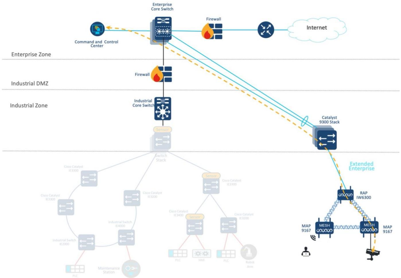
Catalyst Center does not yet support intent-based network automation to enable the Ethernet bridging solution. For this profile validation, Catalyst Center CLI templates are used to enable the required configurations. For enabling the Ethernet bridging solution in Cisco Catalyst 9800 Wireless Controllers, see [Cisco Catalyst 9800 Series Wireless Controller Software Configuration Guide](#).
