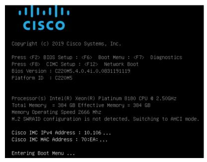
Step 3 Choose the ISO boot drive from the Cisco IMC Mapped DVD (tested), USB flash drive (not tested), or KVM Mapped DVD (not tested).
