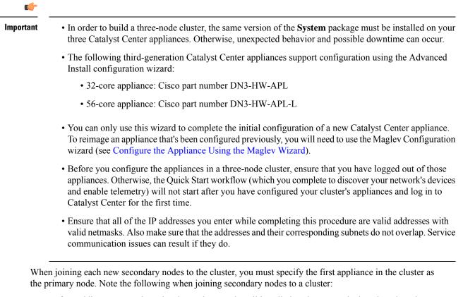
• Before adding a new node to the cluster, be sure that all installed packages are deployed on the primary node. You can check this by using Secure Shell to log in to the primary node's Catalyst Center Management port as the Linux user (*maglev*) and then running the command maglev package status. All installed packages should appear in the command output as DEPLOYED.
