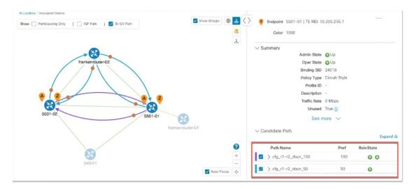
When the Active path goes down, the Protected path immediately becomes "active". When the Active path goes back up, then the Protected path takes the role of "protected" again and the Active path (with preference 100) becomes active.
