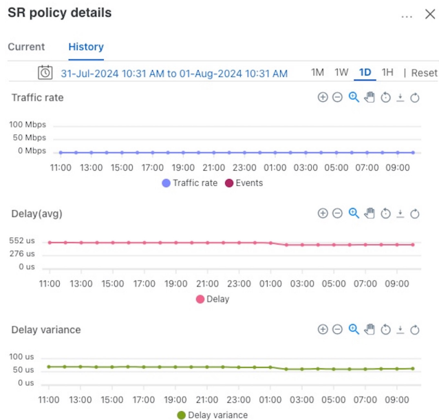
Figure 3: Example of VPN service when monitoring is enabled
