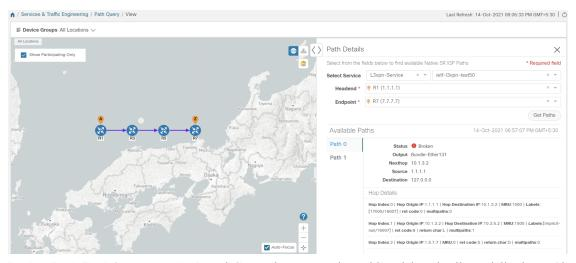
**c. Broken Path (Path is not complete):** Path Status shows as Broken with path hop details partially shown (depending on gNMI output for traceroute – see Step 17 for troubleshooting details) and overlay details partially shown. An Error message will appear indicating that the devices and links are not available.
