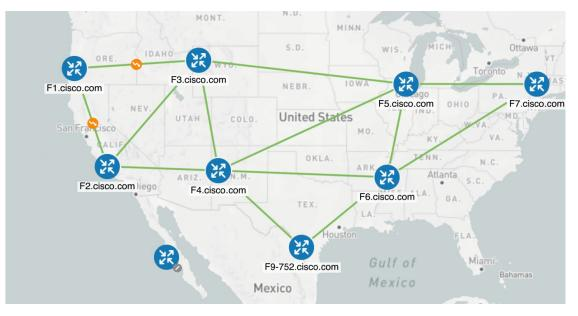
We will enable LCM with a configuration that results in the link between **F3.cisco.com** and **F5.cisco.com** becoming over-utilized. We will then review the mitigation solutions Crosswork calculates. In this example, it is left to the operator to choose to apply the solution.
