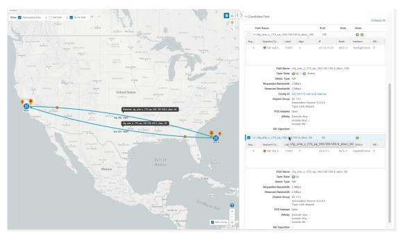
c) Here is a closer view of an Active path's configuration details. Notice that it is designated with the "A" icon under State to indicate that it is currently the operational Active path. Also, if the policy configuration was done through Cisco Crosswork, you have the option to view the policy configuration. To see the configuration, click the link next to Config ID.
