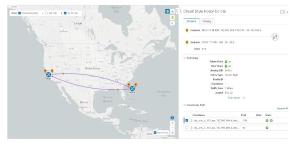
Here is a closer look at the types of Summary details available to you. The **Candidate Path** list at the bottom of the window displays the Active and Protected paths. The Active path is the one that currently takes traffic.
