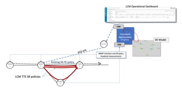
Assuming you deploy these TTE SR policies, LCM continues to monitor the deployed TTE policies and will recommend modifications or deletions as needed in the LCM **Operational Dashboard**. TTE SR policy removal recommendations will occur if the mitigated interface would not be congested if these policies were removed (minus a hold margin). This helps to avoid unnecessary TTE SR policy churn throughout the LCM operation.
