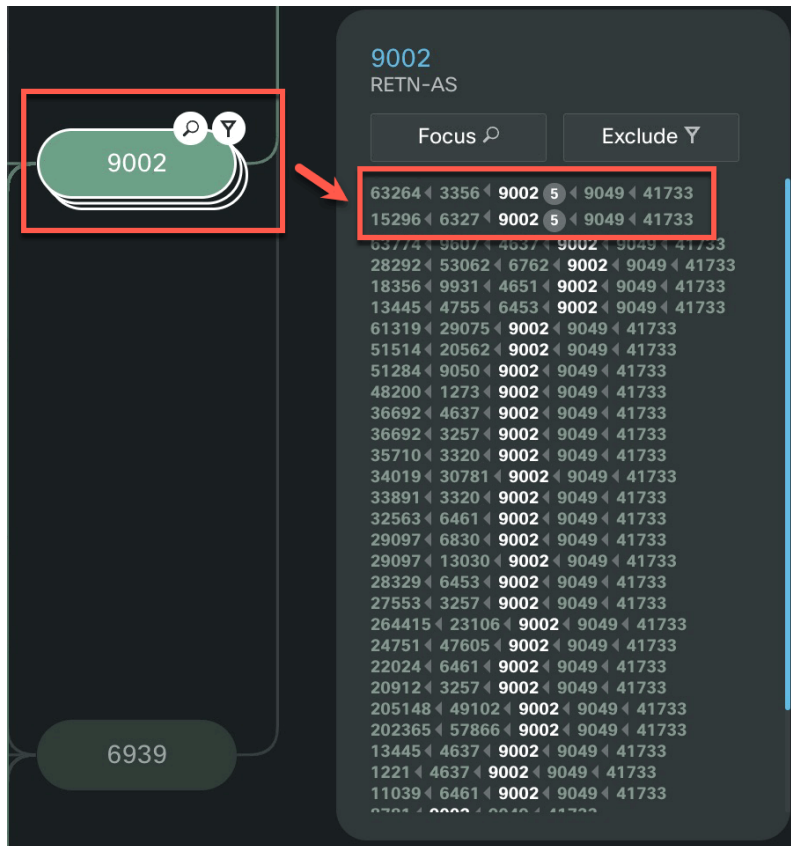
Figure 2: ASN Path Stuffing (ASN Path Prepending) Example
