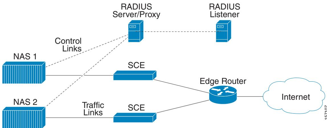
To solve the problem of distinguishing between two NAS devices, the following algorithm is used:
