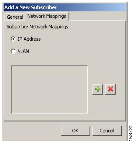
The system supports either IP addresses or VLAN tags as network identification for subscribers.
