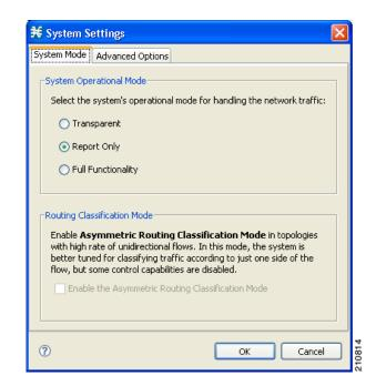
Step 2 Select one of the System Operational Mode radio buttons:
