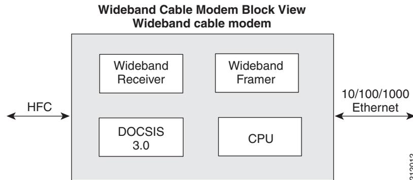
The wideband cable modem has a wideband receiver that receives the multiple RF channels of a bonded channel. It also has a wideband framer that decodes the signal from the wideband receiver and extracts the packets for the 10/100/1000-Mbps Ethernet home network.
