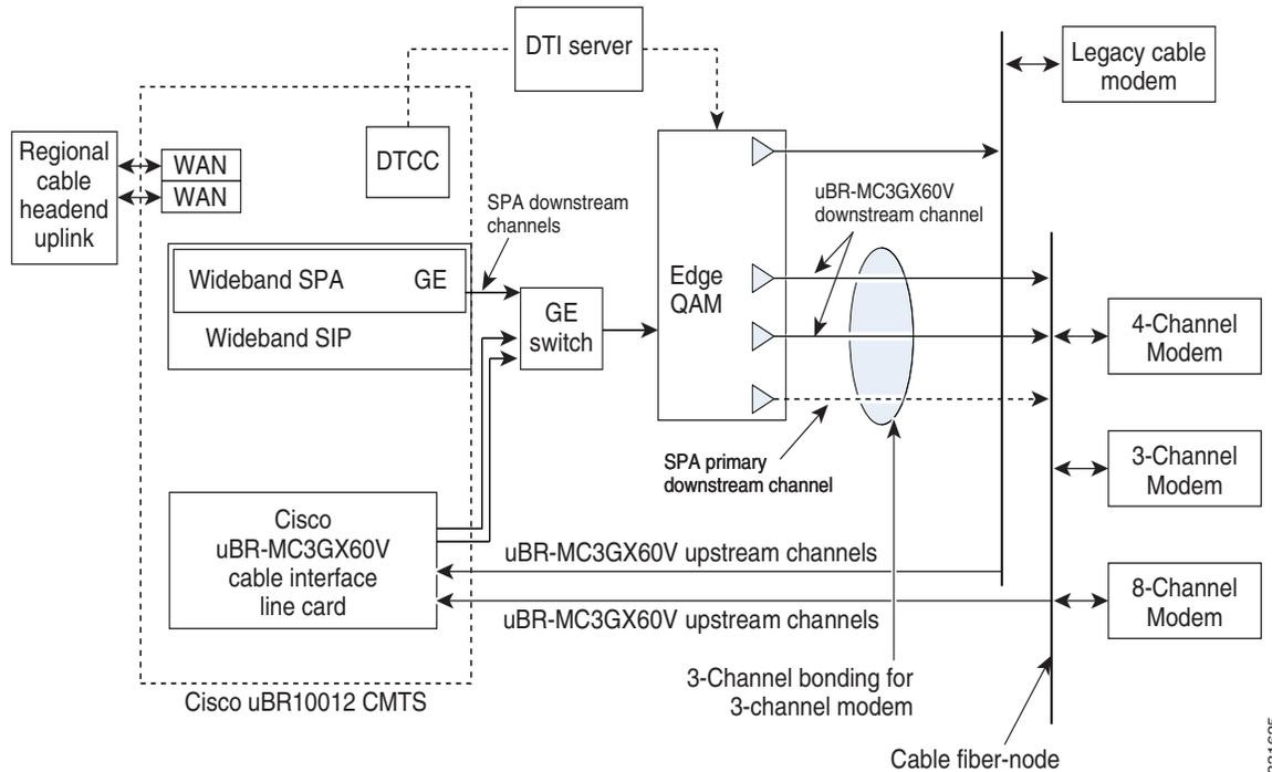
In the M-CMTS architecture used for the Cisco DOCSIS 3.0 DS Solution, traditional Cisco CMTS functionality is divided into three network elements and an interface, as specified below:
