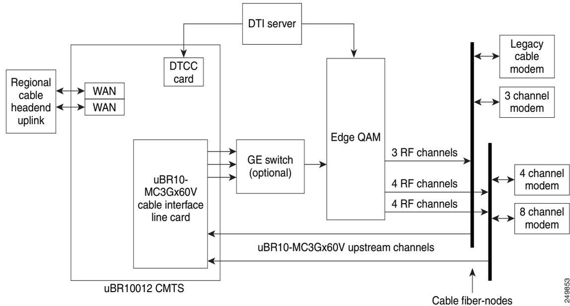
Figure 5-2 shows the M-CMTS architecture used in the Cisco DOCSIS 3.0 DS Solution, with a single wideband channel. In this example, three DS RF channels are bonded together into one wideband channel. The GE switch is optional. The Wideband SPA Gigabit Ethernet Interface can be connected directly to the GE Interface on the Edge QAM.
