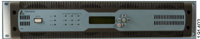
Figure 2-13 Harmonic NSG 9000 Edge QAM Device
