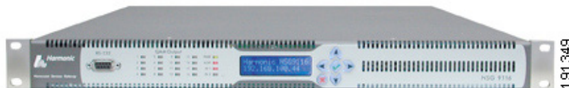
Figure 2-12 Harmonic NSG 9116 Edge QAM Device
