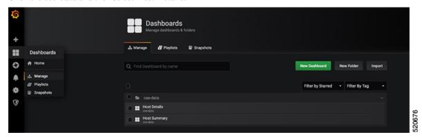
**Step 5** To view details of CPU, Memory, or Disk usage, select the **Host** on the top left corner of the screen.
