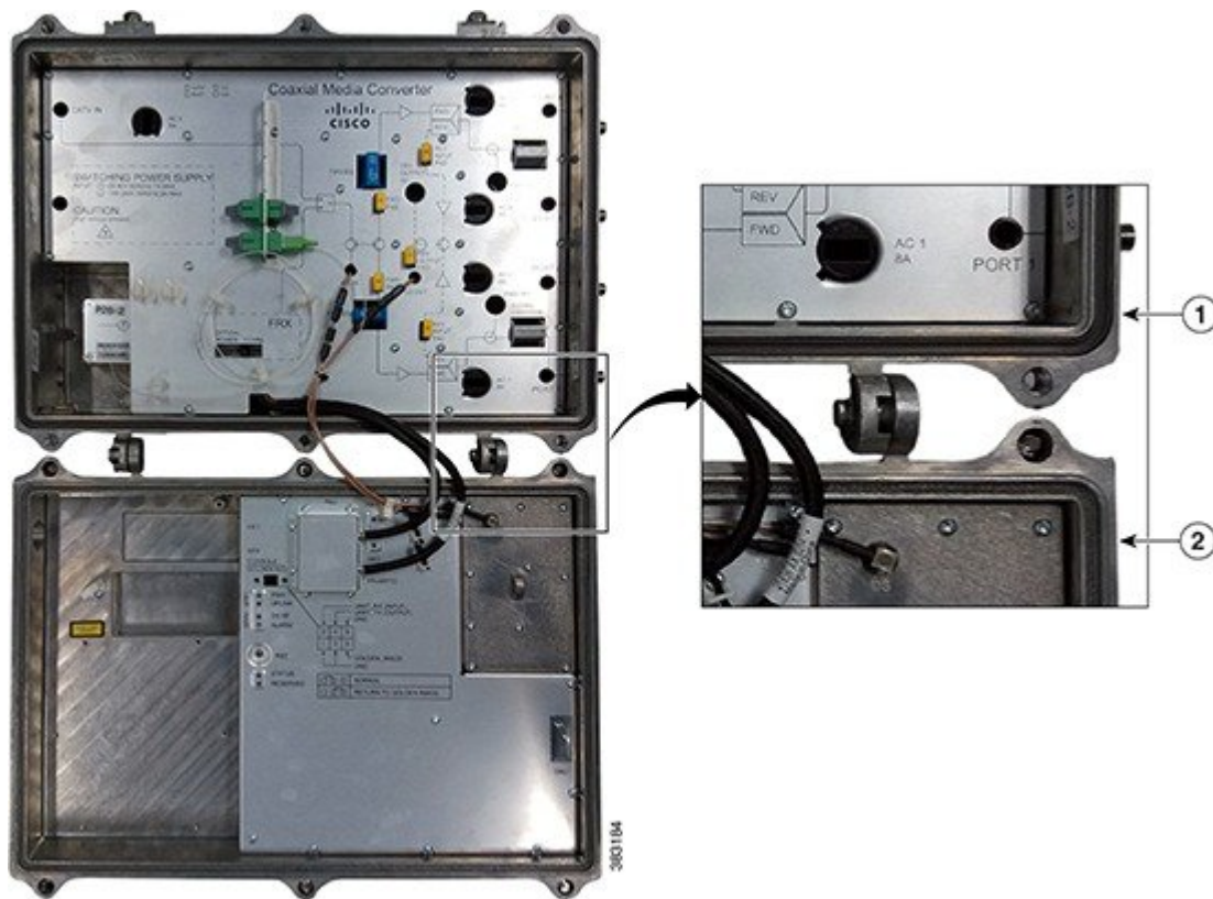
Figure 25: Location of the Waterproof Rubber and EMI Gasket on the Cisco CMC
