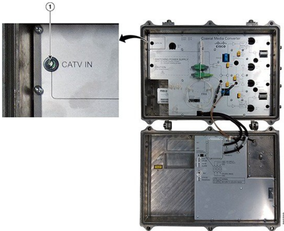
Figure 3: Location of the Seizure Screw
