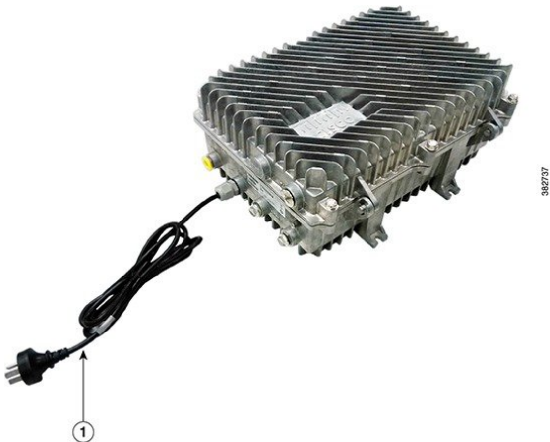
Figure 21: Connecting 220VAC Power to the Cisco CMC
