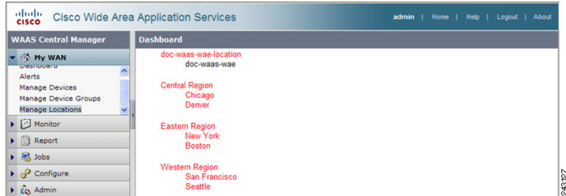
Figure 3-3 Example of the Location Tree
