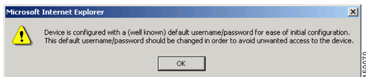
Figure 6-1 Message Indicating the Predefined Password for the Superuser Account Should Be Changed
