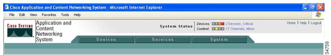
The system status reporting mechanism uses four alarm lights to identify problems that need to be resolved. Each light represents a different alarm level, as follows:
