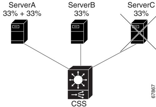
[Figure 13-7](#) shows three cache services configured for **failover linear** (the default). If you suspend ServerB or if it fails, the CSS does not rebalance the services. It evenly distributes ServerB cache workload between servers A and C.
