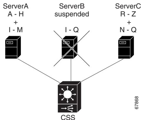
Figure 13-8 also shows three cache services configured for failover **linear**, but in this example, you remove ServerB using the **remove service** command from owner-content mode. Because the CSS does not apply the failover setting when you remove a service, it rebalances the remaining services.
