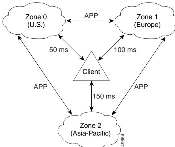
In [Figure 5-1](#), the lowest RTT value is returned from Zone 0. Therefore, Network Proximity would link the client to a service located in Zone 0, regardless of the physical location of the client. The three zones communicate with each other using the Application Peering Protocol (APP). For details on APP, refer to [Chapter 1, Configuring the CSS Domain Name Service](#), in the section “[Configuring Application Peering Protocol](#)”.
