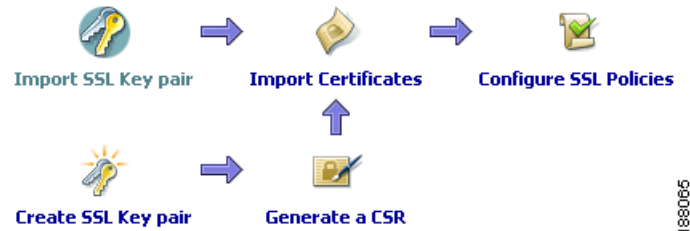
Figure 11-2 SSL Setup Sequence
