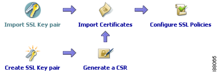
Figure 10-2 SSL Setup Sequence
